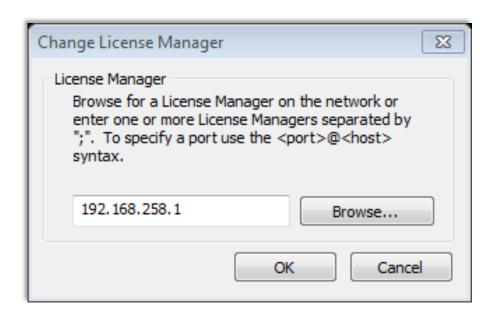
5 You can find the IP address of the Licence Manager by running the command IPONFIG in the command window, and copying the IPV4 address.
